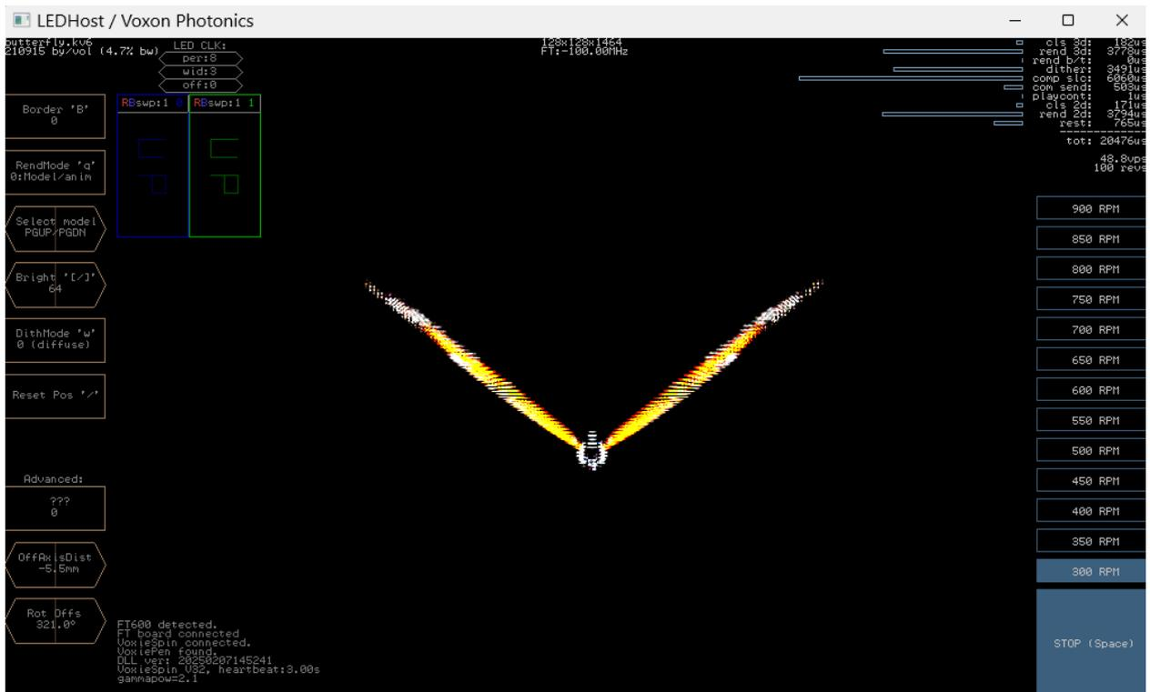
**At any time, press Space, or the STOP button in the lower right of the LEDHost window to stop the display motor.**
